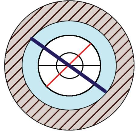
Red Line - Diameter of Gas Burner (White Circle) Blue Line - Fire Pit Opening Diameter (Lite Blue Circle) Grey Cross Hatch -- Outer Ledge of Pit
